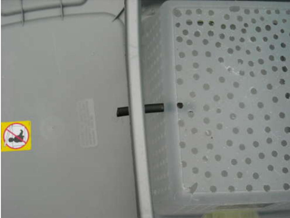
It is important to put your drain hole at the top of where your water line should be. So put it at the top of the basket. A simple hole in the side will clog with dirt a little and drain slower, so I used a small rubber auto hose to "bring" my drain hole inside the basket as pictured. Try to make the hole in the side the same size as your drain hose but there is no reason to make it a perfect fit or seal it of...lol... it's a drain! :)
