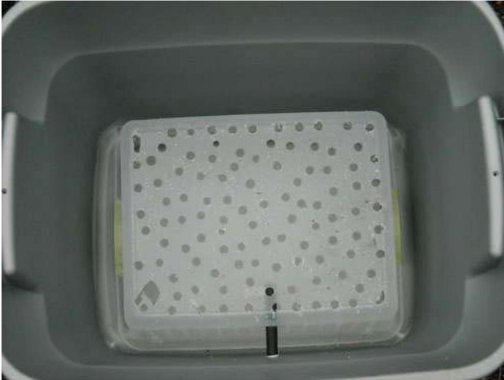
Drill holes all throughout the bottom of your basket I'd say anything between a 1/4" and 3/8" are good... I used a step bit so mine came out random sizes.
